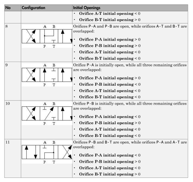
The other nine configurations are covered by the remaining 4-way directional valve blocks (A through K), as shown in the next table.
