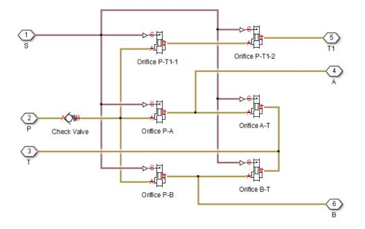
All the orifices in the model are closed (overlapped) in valve neutral position, except orifices  $P_{1_1}$  and  $P_{1_2}$ . These two orifices should be set open to an extent that allows pump delivery to be discharged at low pressure.
