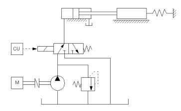
The power unit consists of a motor, a positive-displacement pump, and a pressure relief valve. Depending on its characteristics, such a power unit can be modeled in a variety of ways, as described in "Modeling Power Units" on page 2-27. In this example, the pump unit is assumed to be powerful enough to maintain constant pressure at the valve inlet. Therefore, we are going to represent it in the diagram by a Hydraulic Pressure Source block.
